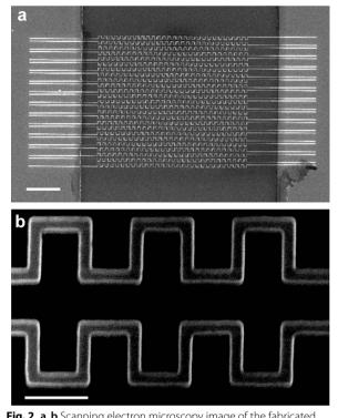
**Fig. 2** a, b Scanning electron microscopy image of the fabricated nanowire pattern on SOI wafer. (Scale bar a 5  $\mu$ m; b 500 nm)
