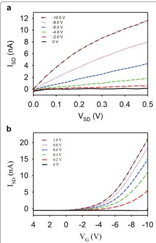
**Fig. 3** Electrical properties of silicon nanowire-based FET device. **a** Source–drain current ( $I_{SD}$ ) versus source–drain voltage ( $V_{SD}$ ) plots at different gate voltages. **b** Source–drain current ( $I_{SD}$ ) versus gate voltage ( $V_{C}$ ) at a different source–drain voltage ( $V_{SD}$ ) of the fabricated nanowire pattern on SOI wafer
