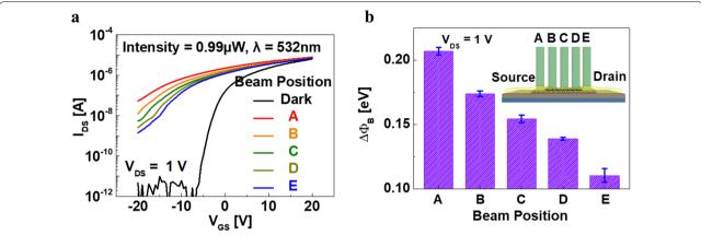
**Fig. 5**  $a \mid_{DS} - V_{GS}$  curves and b variations in the barrier height with the beam position of the multi-layer MoS<sub>2</sub> phototransistors (Inset: 3D schematic image of a MoS<sub>2</sub> phototransistor representing the different beam positions)
