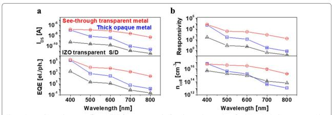
**Fig. 4** a  $I_{Photo}$  and external quantum efficiency (EQE), **b** responsivity and collected carrier density values of multi-layer MoS<sub>2</sub> phototransistors with see-through metal, thick opaque metal and IZO transparent metal electrode under illumination at different wavelengths
