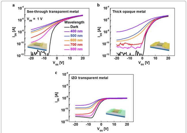
**Fig. 3**  $I_{DS}$ – $V_{GS}$  characteristics of the multi-layer MoS<sub>2</sub> phototransistor with **a** see-through metal, **b** thick opaque metal and **c** IZO transparent metal in the dark and under illumination at different wavelengths
