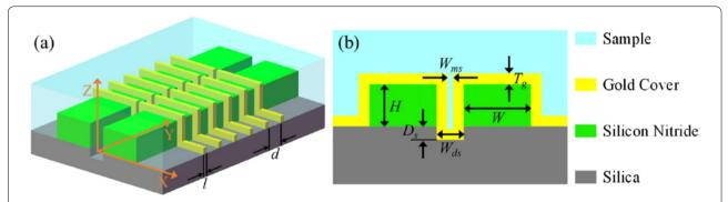
Fig. 7 a Schematic diagram of the SERS sensor based on the hybrid plasmonic grating slot waveguide. **b** Cross section of the hybrid plasmonic slot waveguide. (Reprinted with permission from Ref. [58])
