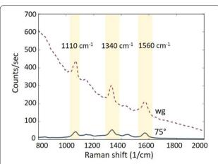
**Fig. 17** The dashed curve is the measured back-scattered Raman spectrum with the waveguide mode excitation. The solid curve is the spectrum obtained for an oblique free-space excitation at an angle of 75°. The NTP Stokes peaks are highlighted by yellow shaded areas. Adapted with permission from Ref [65], Copyright © 2020, IEEE
