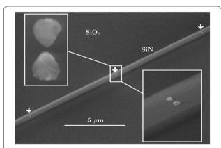
**Fig. 10** Scanning electron microscope image of a functionalized waveguide. The white arrows indicate antenna positions. The insets show a zoom of a typical antenna. (Reprinted with permission from Ref. [60])
