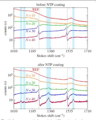
**Fig. 11** Raman spectra, before and after NTP coating, of a reference waveguide (N = 0) and waveguides functionalized with N = 10, 20, 30, 40 antennas. (Reprinted with permission from Ref. [60])
