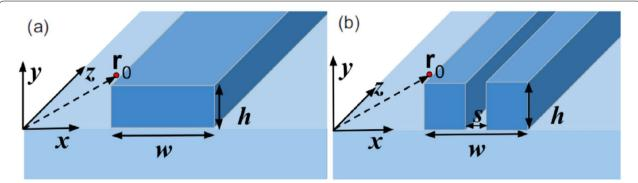
**Fig. 2** Schematic of a dielectric **a** strip and **b** slot waveguides defined by a core of higher refractive index ( $Si_3N_4$ ,  $TiO_2$  or silicon) patterned on a lower index bottom cladding (typically silicon dioxide). The scattering particles are assumed to be embedded with a uniform density in the upper cladding (colorless region). A particle at position  $\mathbf{r}_0$  is shown for both cases. (Reprinted with permission from Ref. [54])
