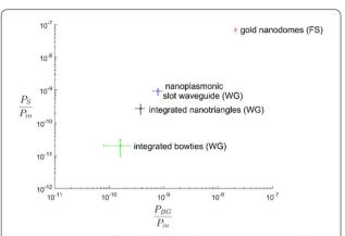
**Fig. 13** Comparison of SERS background power  $P_{BG}$  (x-axis) and SERS Stokes power  $P_S$  (y-axis) of different SERS platforms. Both parameters are normalized on the input power and the integration time. FS indicates free-space and WG is the waveguide-based excitation. (Reprinted with permission from Ref. [62])
