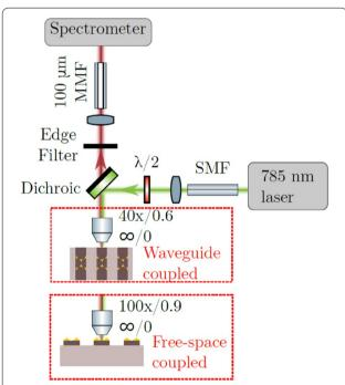
**Fig. 8** Schematic of the confocal microscope used for collecting Stokes scattered light from both waveguide- and free-space coupled nanotriangles. (Reprinted with permission from Ref. [59])
