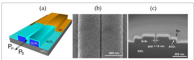
Fig. 15 Nanoplasmonic slot waveguide. a Schematic showing that the input and Stokes powers are guided by the waveguide. b Scanning electron microscope image of the gold-covered slot in top view. c Cross-section of a nanoplasmonic slot waveguide with a gap. Reprinted with permission from Ref. [64]
