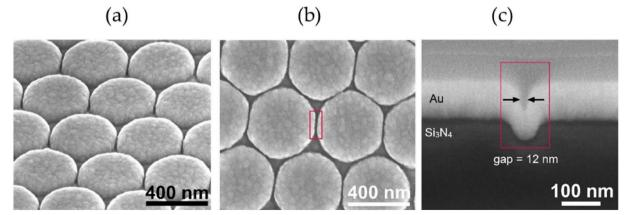
Fig. 12 Scanning electron microscope images of gold nanodomes. a Tilted view. b Top-down view. c Cross-section of a nanodome-patterned chip with a 12 nm wide gap between nanodomes. (Reprinted with permission from Ref. [62])
