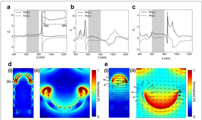
Fig. 4 Effective optical parameters and electrical field diagrams of SSRR under *x*-polarized light. Effective **a** wave impedance, **b** permittivity, and **c** permeability of SSRR. **d** Electric and **e** magnetic field profile of SSRR at λ = 550 nm and 837 nm, respectively. (i) *x*–*z* cross-section and (ii) *x*–*y* cross-section of SSRR
