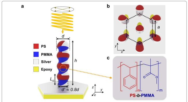
**Fig. 1** Schematic of stacked split-ring resonators (SSRR). **a** Tilted view of a SSRR and geometric parameters (d and d'the diameter of PS and PMMA nanodomains, respectively, h: the height of nanorod). **b** Top-view of a hexagonal array of SSRR (a: the center-to-center distance between two neighboring nanorods). **c** Chemical structures of PS-b-PMMA
