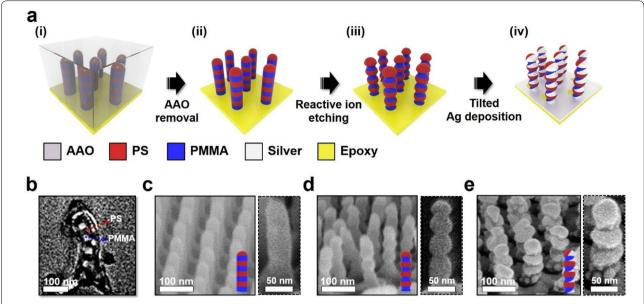
**Fig. 2** Fabrication of a high-density array of stacked split-ring resonators (SSRR). **a** Schematic of fabrication of SSRR nanostructures. TEM image of **b** stacked lamellae. FE-SEM images of **c** the stacked lamellae nanorods, **d** pagoda-like nanostructures, and **e** stacked split-ring resonators (the brighter part is Ag and the darker part is PMMA block). Dotted boxes in **c**-**e** are expanded images
