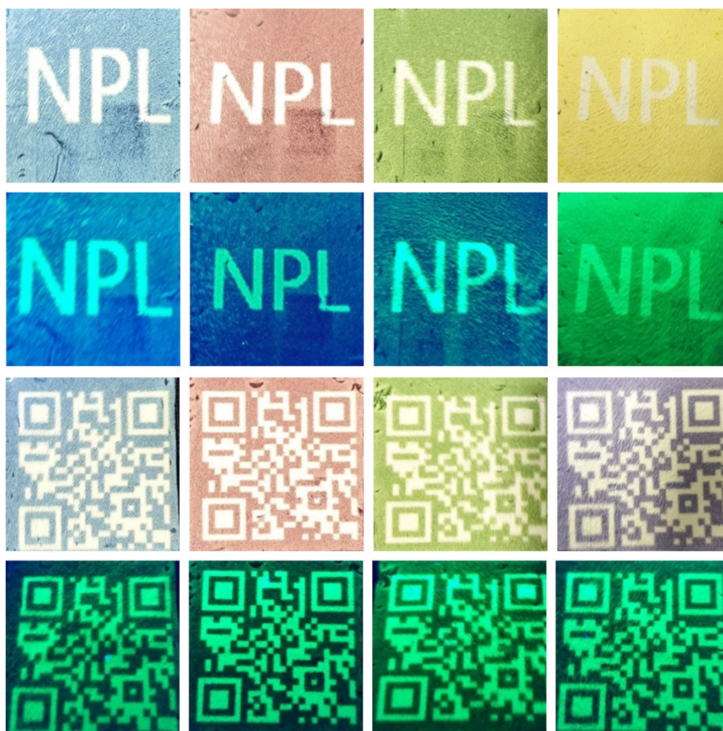
Fig. 4 Anti-counterfeiting application. Alphabet “NPL” and QR code patterns printed with blue, brown, green, and yellow on an inkjet printer using a reverse printing approach on fluorescent PCL-perovskite fibers-based white paper
