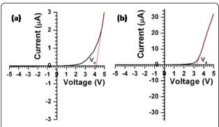
Figure 8 Current versus voltage plots of (a) untreated (D1) and (b) treated ZnO NRs (D2) based p-n junction diodes.
