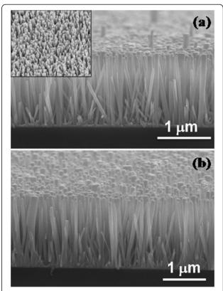
Figure 1 Cross sectional FESEM images of (a) as-grown and (b) plasma treated (20 min) ZnO NRs (inset of Figure 1a shows the surface morphology of as-grown ZnO NRs).
