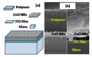
Figure 7 (a) Schematic diagram and (b) cross-section FESEM images of ZnO NRs/polymer based p-n junction diode.
