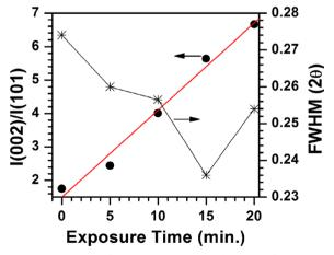
Figure 3 Variation of I(002)/I(101) ratio and FWHM of ZnO NRs as a function of plasma exposure time.
