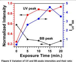
Figure 5 Variation of UV and BB peaks intensities and their ratio  $(I_{UV}/I_{BB})$  of ZnO NRs as a function of plasma exposure time.
