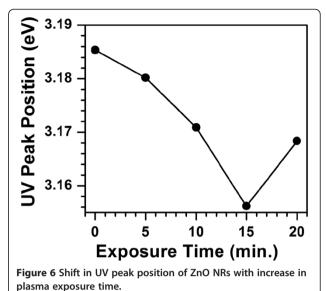
interstitials  $(Zn_i)$  under moderate temperatures [31]. The newly formed Zn-N phase and/or regenerated oxygen interstitials probably leads the band gap of ZnO NR structures to slightly higher values. Therefore, the structures exposed to nitrogen plasma for 15 min duration consist of better crystallinity as well as optical quality and thus, these structures are adopted for the development of p-n junction diodes.
