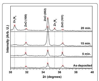
Figure 2 XRD profiles of as-grown and plasma treated ZnO NRs for the three typical exposure timings of 5, 15 and 20 min.
