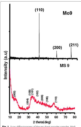
**Fig. 1** X-ray diffractograms of the resultant powder samples, Mo9 and MS9
