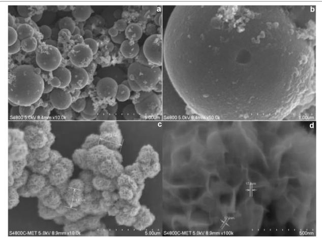
Fig. 2 FESEM images of the sample Mo9 under **a** low-magnification **b** high-magnification and sample MS9 under **c** low-magnification and **d** high-magnification
