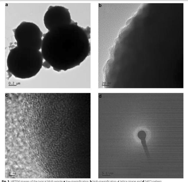
Fig. 3 HRTEM images of the typical Mo9 sample a low-magnification, b high-magnification, c lattice image and d SAED pattern
