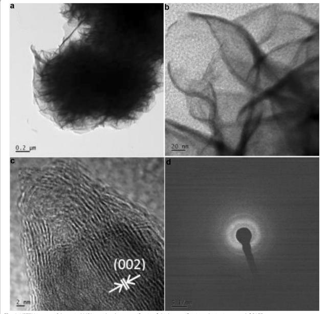
Fig. 4 HRTEM images of the typical MS9 sample **a** low-magnification, **b** high-magnification, **c** lattice image and **d** SAED pattern
