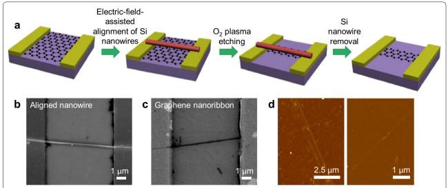
**Fig. 4** a Schematic illustration of the fabrication of a GNR FET using a Si NW as a hard etch mask. FESEM images of **b** a Si NW aligned on graphene between two electrodes, where unscreened graphene was removed, and **c** a GNR after the removal of the Si NW. **d** AFM images of GNRs with two different ribbon widths (left: 500 nm and right: 100 nm)
