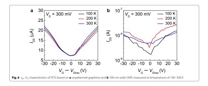
the GNR. These results demonstrate the opening of the bandgap in graphene due to enhanced carrier confinement in the transverse direction and the edge effect in the ribbon structure.
