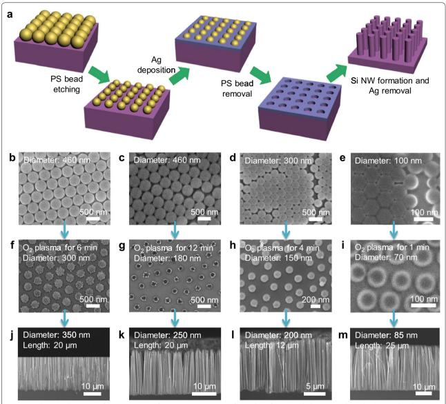
**Fig. 2** a Schematic illustration of the preparation of a Si NW array using a Ag film with uniform-sized holes as an etch mask, where PS beads were used for patterning the Ag film. **b-m** FESEM images of the process steps for fabricating vertically aligned, ordered Si NW arrays
