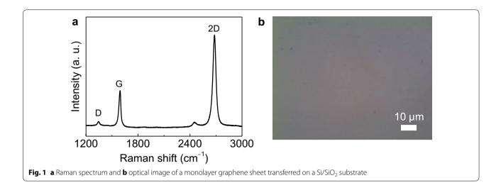
graphitic carbon species, the intensity of which was associated with the level of defects in the crystalline structure of the graphene layers. This weak D band confirmed the high quality of the synthesized graphene films. Figure 1b shows an optical image of the uniform graphene sheet transferred on a  $SiO_2$  layer.
