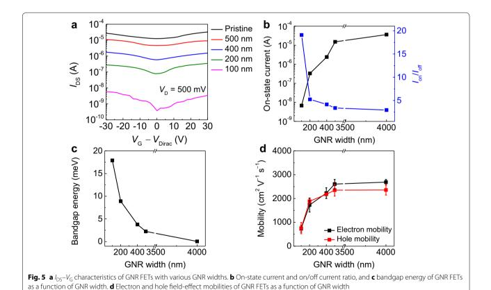
ratio is inversely proportional to GNR width, e.g., the on/off current ratio for 500-nm wide GNR FETs is only 3.5 but gradually increases to 20 with decreasing ribbon width to 100 nm. This trend was consistent with previous
