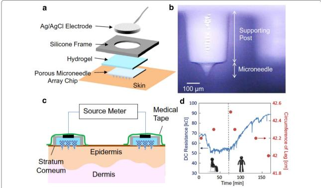
**Fig. 4** a Schematic of the porous MN-based intercellular swelling measurement system. **b** A micrograph of the porous PEG MN. **c** Schematic of the DC resistance measurement by two porous MN array. **d** The DC resistance measured by the porous MN array and the circumference changed by a movement (Reproduced with permission [110]. Copyright 2015, Springer Science + Business Media, LLC)
