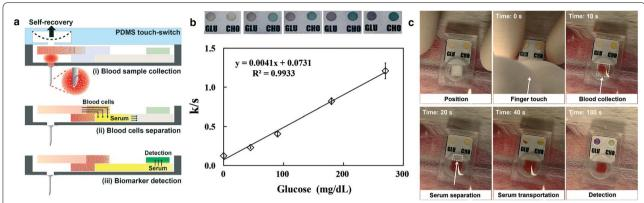
**Fig. 3** a The sampling and measurement process of blood using a hollow MN and paper-based sensor. **b** The change of color (above) and calibration curves for glucose measurement (below). **c** A series of optical images of the blood sampling and glucose measurement in a rabbit ear with the integrated hollow MN and the paper-based sensor (Reproduced with permission [89]. Copyright 2015, the Royal Society of Chemistry)
