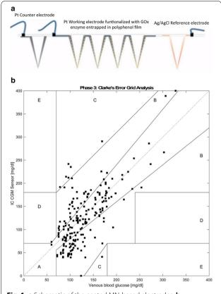
**Fig. 1** a Schematic of the coated MN-based electrodes, **b** Measurement of Clarke error in the 24 h clinical test of the glucose monitoring system with the MN array (Reproduced with permission [52]. Copyright 2018, the Royal Society of Chemistry)
