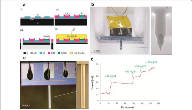
**Fig. 2** a Cross-sectional fabrication process of the electrodes on the Si MN. **b** An optical image of the assembled hollow MN and measurement setups. SEM image of the hollow MN is shown on right hand, **c** A micrograph of the fabricated electrodes on the Si probe, **d** Amperometric measurement of glucose by the hollow MN-based sensor (Reproduced with permission [66]. Copyright 2018, IEEE)
