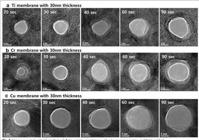
Fig. 2 Nanopore evolution for 30 nm thick a Ti, b Cr, and c Cu membranes with e-beam exposure time, at 200 kV and 7 nA
